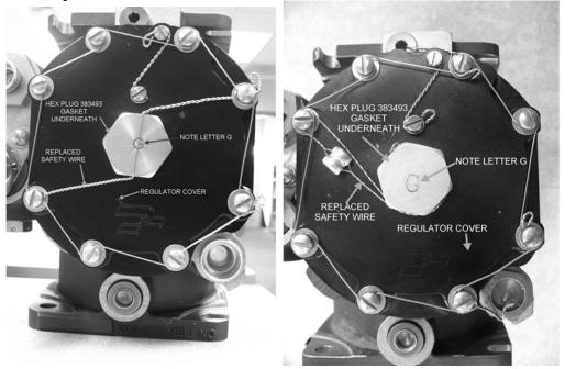
Note: The safety wire through the hex plug shown in the left hand photo is .025" wire wrapped around regulator screws under existing wire. It does not go through the holes in the screws. The safety wire through the hex plug shown in the right hand photo is .015" wire which passes through the regulator screw hole. This is the normal safety wire method used at the factory.
